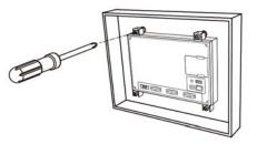
Mount the HMI according to the illustration below. Incorrect installation direction may result in
